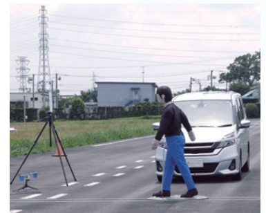
Experiment of advanced emergency braking system
