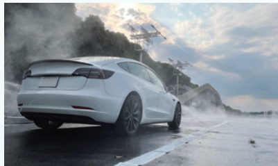
Evaluation experiments on automated vehicles' environment recognition performance in the rain
