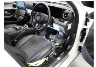
Automatic acceleration and braking system developed by NTSEL
