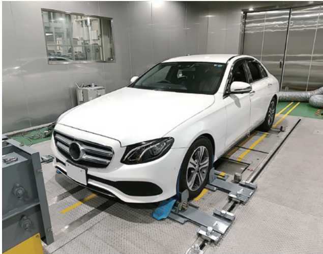
Environmental performance evaluation under low-temperature environment
