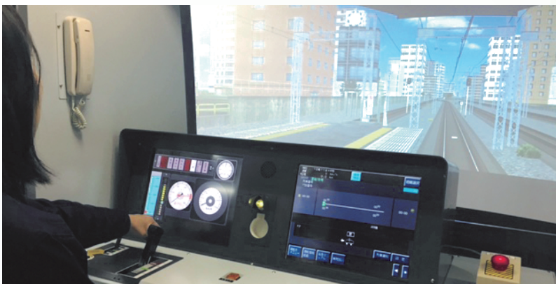
Train operation safety evaluation simulator (driver's cab)
