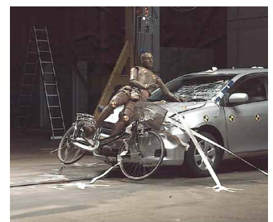
Collision experiment between a passenger vehicle and a cyclist
