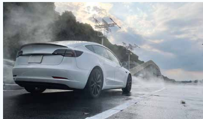
Evaluation experiments on automated vehicles' environment recognition performance in the rain
