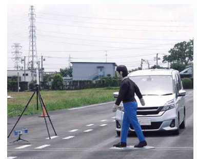
Experiment of advanced emergency braking system
