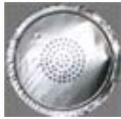
PM Deposition on 1 st stage of ELPI (50% Cut off dia. 30 nm)
