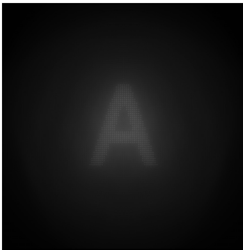
(b) Optical depth : 8 , Mean particle radius : 3 μm Lighting of character portion
