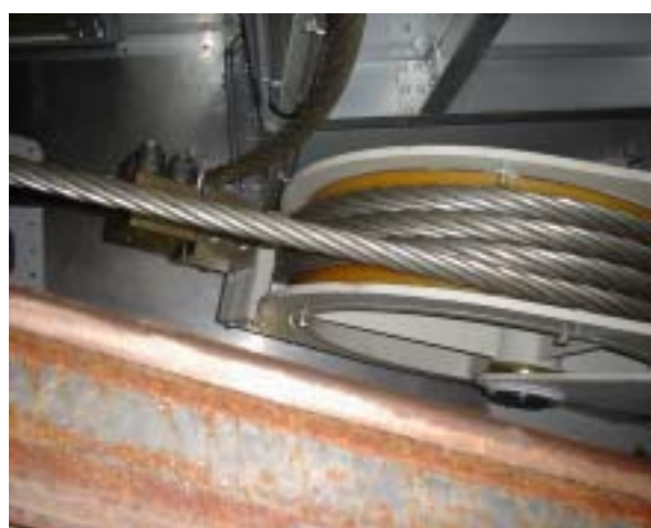
Fig.2 Haul rope attachment device (Rope drum)
