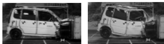
Fig.30. Photos of overload test (Minicar B)
