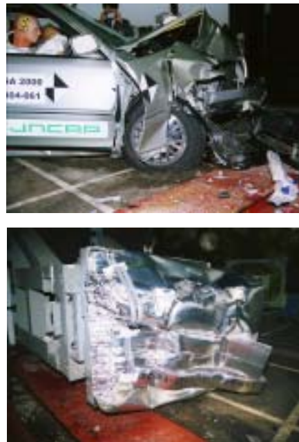
Fig.24. Car and barrier deformation in a 64 km/h ODB test.
