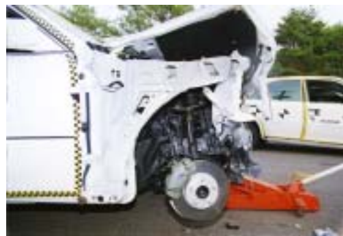
Fig.10. Car deformation in full rigid barrier test
