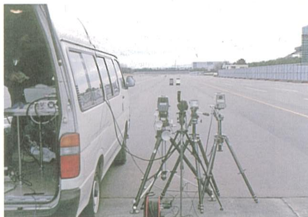
Fig.10 Scene of measurement of the ambient luminance distribution by using CCD camera
