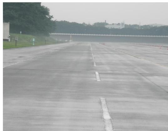
Figure 5, Test track of light wet condition that increases 15 % of rolling resistance
