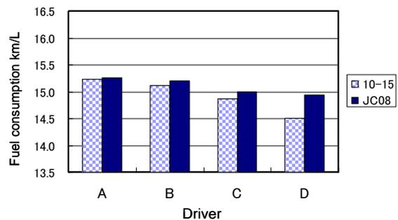
Figure 19, Fuel consumption for each driver at 10-15 and JC08 test cycle
