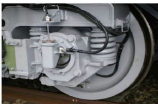
(a) Sensor for wheel load
