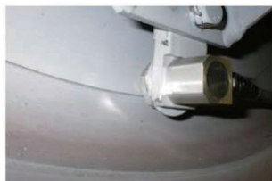
(b) sensor for lateral force
