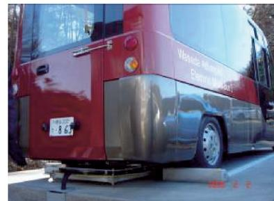
Fig. WEB during Rapid Charging by Non-contact IPS System
