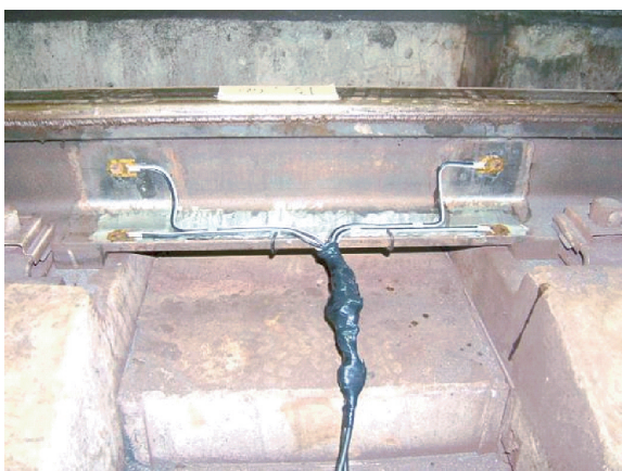
Fig.24 Strain gauges on rail in practical measurement
