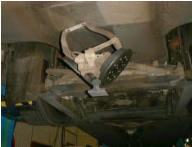
Photo.5 Guide mechanism of Translohr
