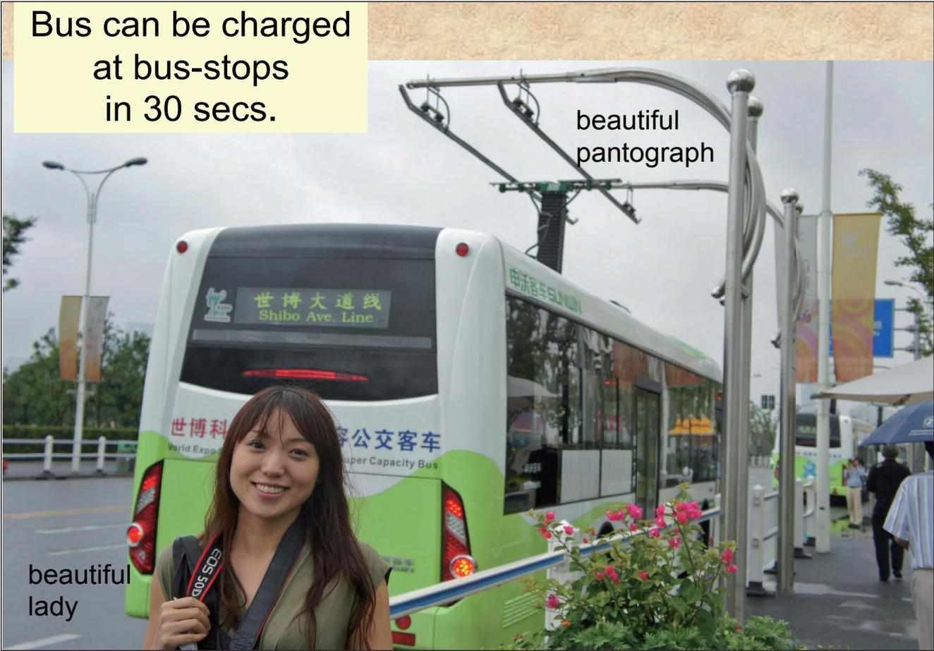
Bus can be charged at bus-stops in 30 secs.
