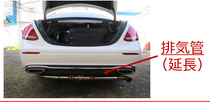
PEMS : Portable Emissions Measurement System
