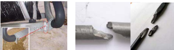
Fig.5 Frame break accident Fig.6 Spring bar break accident
