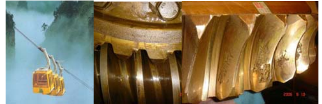
Fig.7 Gearbox damage incident
