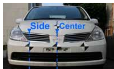
Fig. 8 Impact locations on bumper
