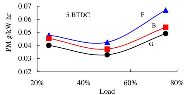
Fig. 11 Emission behavior for different mixture ratios
