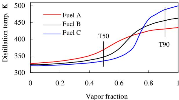
Fig.5 Distillation curves for different ICs
