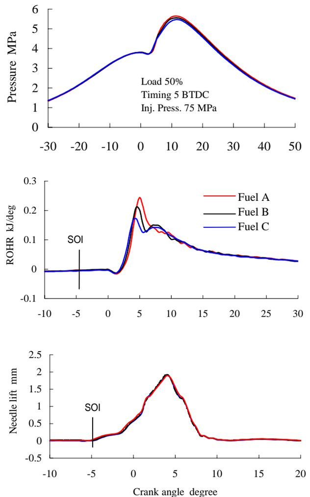
Fig. 4 Combustion behavior for different ICs
