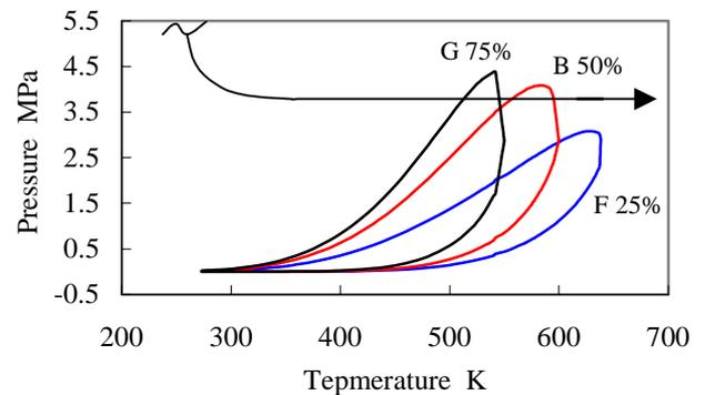
Fig. 10 P-T Diagram for different mixture ratios
