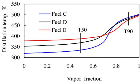
Fig. 9 Distillation curves for different MPC
