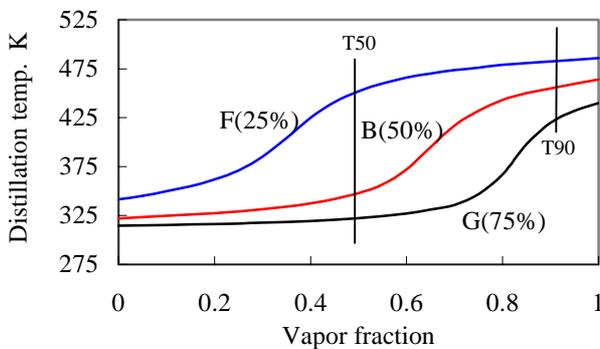
Fig. 13 Distillation curves for different mixture ratios
