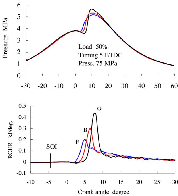
Fig. 12 Combustion behavior for different mixture ratios
