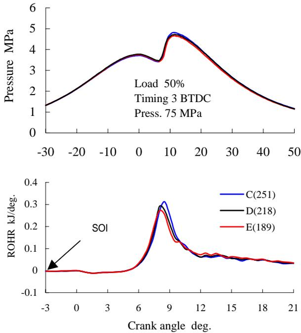
Fig. 8 Combustion behavior for different MPC
