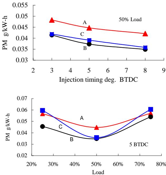
Fig. 3 Exhaust emission for different ICs
