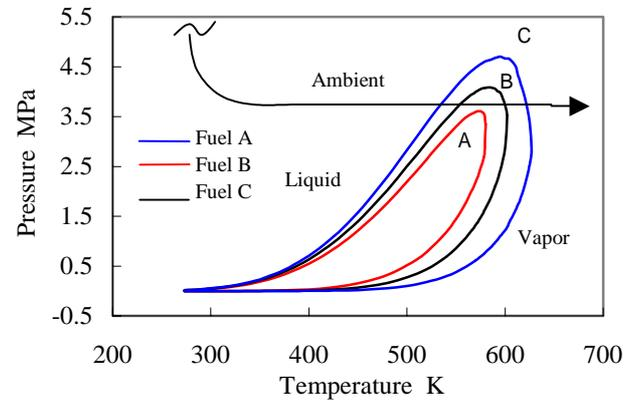
Fig. 2 P-T Diagram for different ICs
