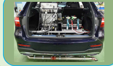
PEMS Portable Emissions Measurement System
