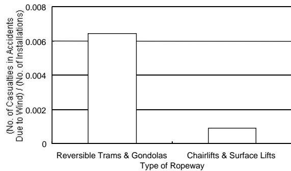
Fig.26 Ratio of "Number of Casualties in Accidents Due to Wind" to "Number of Installations" in Each Type of Ropeway
